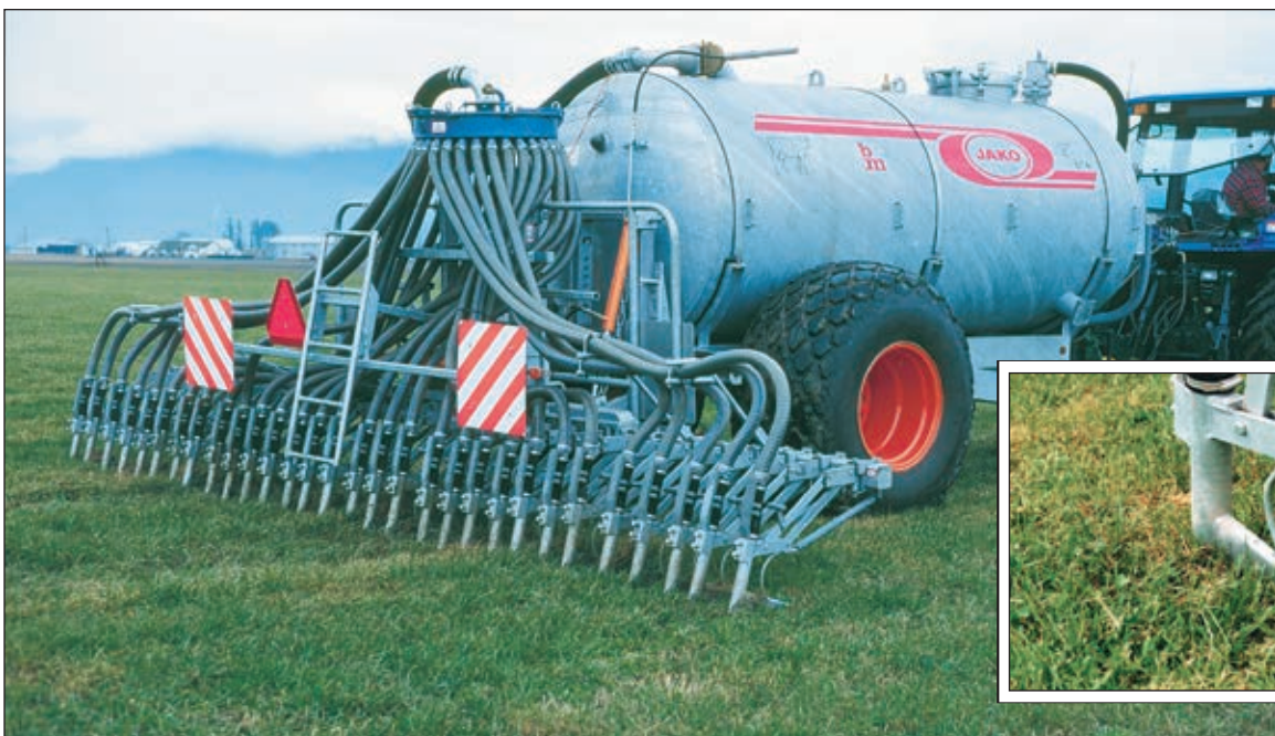
Fig. 11. Banding of manure with the sleigh foot applicator is an effective method of applying slurry on grassland.
