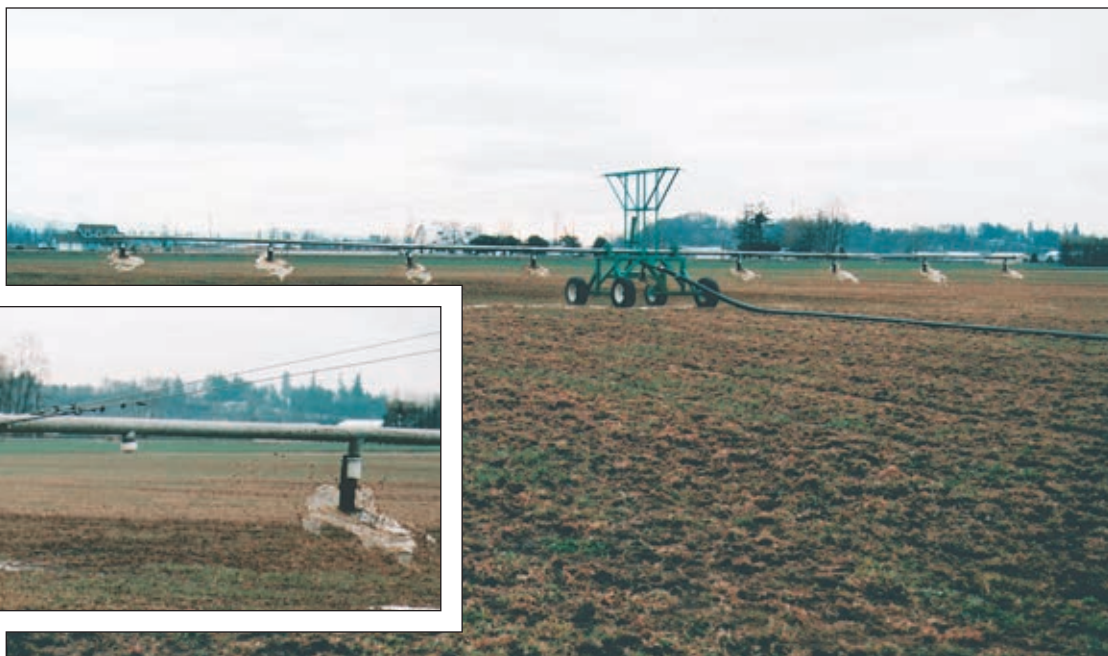
Fig. 14. "Trailing boom" system is a modification of the trailing gun approach (Fig. 13).
