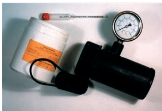
Fig. 22. Nova MKII meter measures ammonium-nitrogen concentration in manure.
