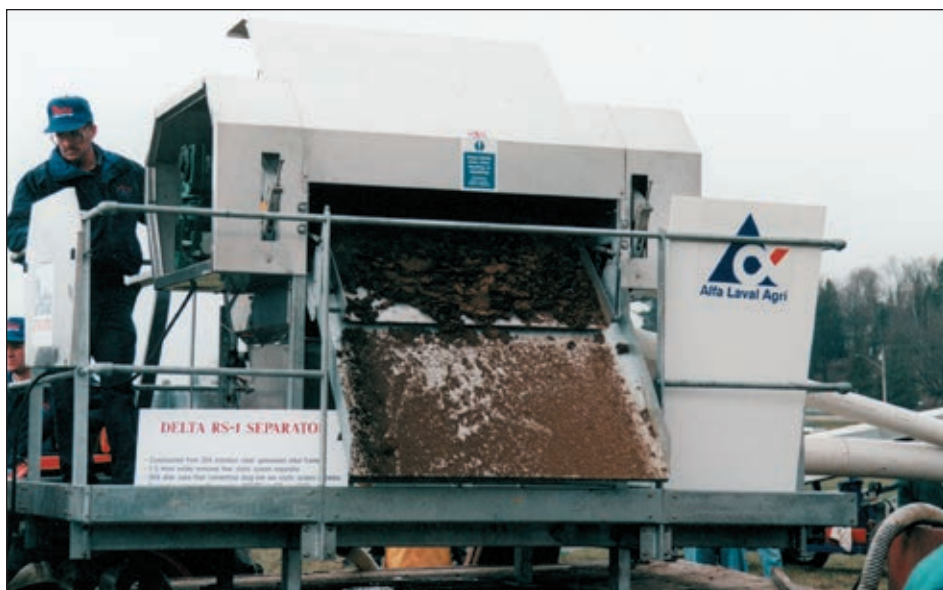
Fig. 9. Separating manure produces a solid fraction high in organic-N and phosphorus and a liquid portion high in ammonium-N and potassium.
