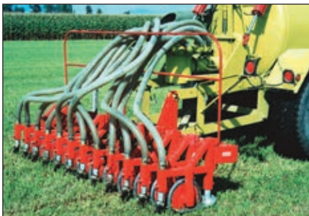
Fig. 10. Shallow injection of manure into sod.
