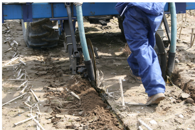
Figure 3: Manure band placement with single disk opener
