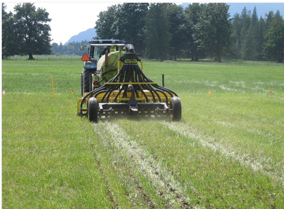
Figure 5. Application of dairy slurry by surface banding over aeration slots created by a rolling tine tool.
