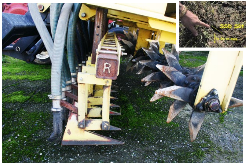
Figure 6. Left: implement for assisted infiltration comprising of the rolling tines and sliding shoe with application hoses attached. This is an adaptation of SSD® implement manufactured by SAPHolland. Inset: Aeration slots formed by rolling tine.
