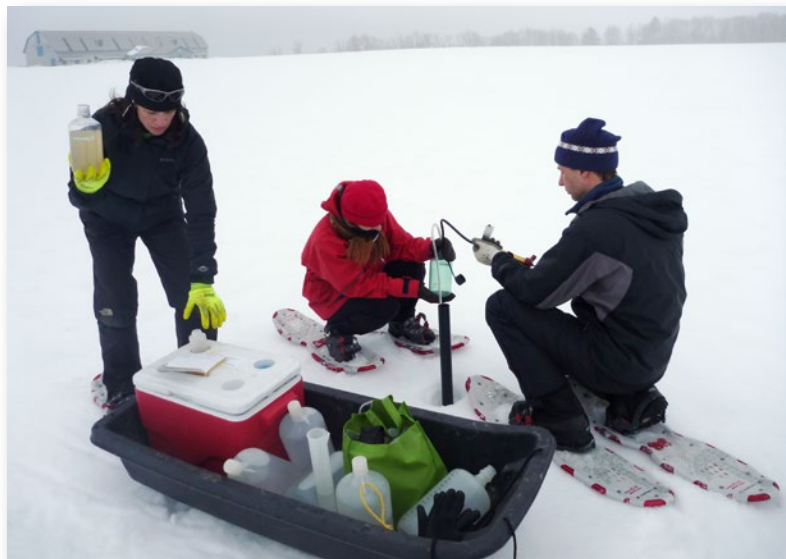
Collecting groundwater samples below the snow cover.
